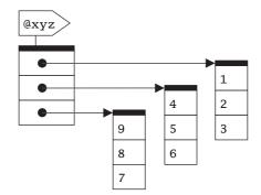
Now, suppose you would like to have just the x (0th) element from each point, as indicated by the shading in the PEGS diagram. You could write a loop using an explicit index, or perhaps a C-style for loop:
